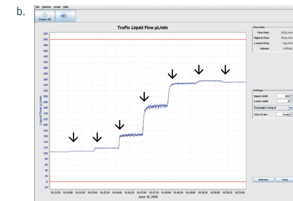
Adjusting pump tension
